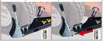
Pedal controlled pneumatically operated main column
