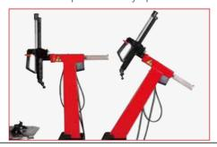
Newly-designed mount/demount foot with a read tab offers significant support during mounting step, Plastic protection inserts are also present to avoid scratching the rims.
