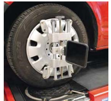
HIGH-RESOLUTION LIGHT TARGET With infrared filter for enhanced immunity to solar reflections.
