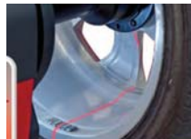
LASERLINE FOR STICK ON WEIGHT
