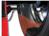
LASERLINE FOR STICK ON WEIGHT
