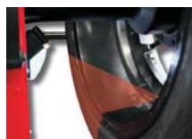
LASERLINE FOR STICK ON WEIGHT
